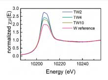
Fig. 5 W  $\mbox{L}_3\mbox{-edge}$  XANES spectra of three W-doped  $\mbox{TiO}_2$  and W-reference samples.
