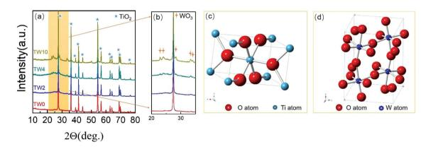
Fig. 2 (a) XRD patterns and (b) magnified XRD patterns in the region of 20-35 degrees of TW0, TW2, TW4 and TW10. (c) TiO<sub>2</sub> and (d) WO<sub>3</sub> unit cell images.
