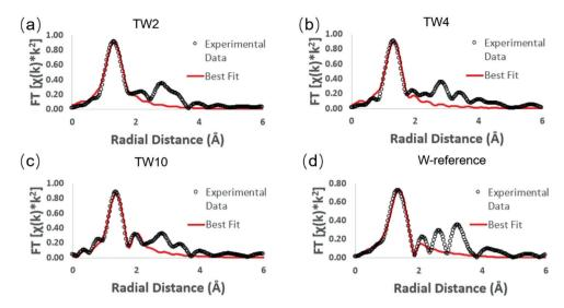
W L<sub>3</sub>-edge FT-EXAFS spectra of different samples: (a) TW2, (b) TW4, (c) TW10, and (d) W-reference.
