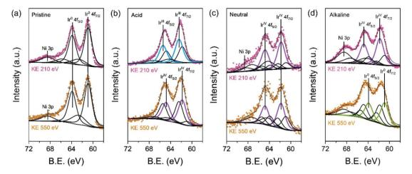
Fig. 4 Electronic structures of electrochemically activated IrNi/C under acidic, neutral, and alkaline conditions. High-resolution XPS spectra for Ir 4f of (a) pristine IrNi/C, (b) IrNiO<sub>x</sub>/C-A, (c) IrNiO<sub>x</sub>/C-N, and (d) IrNiO<sub>x</sub>/C-Al at kinetic energies of 210 eV and 550 eV.
