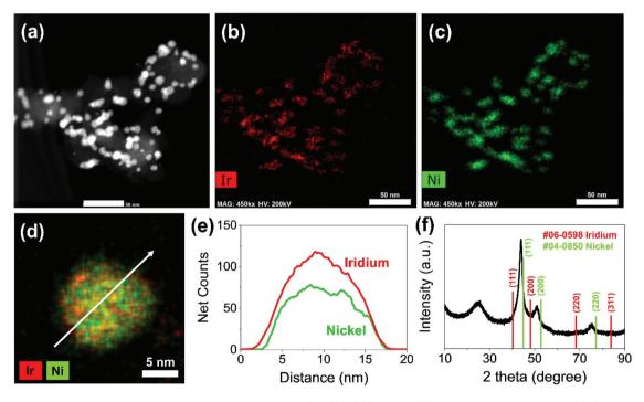
Fig. 1 Morphology of carbon supported IrNi alloy nanoparticles (IrNi/C). (a) HAADF-STEM images of pristine IrNi/C (scale bar: 50 nm). HAADF-STEM elemental mapping analysis of IrNi/C (scale bar: 50 nm): (b) red and (c) green represent Ir and Ni, respectively. (d and e) Line-scan profiles of IrNi alloy nanoparticles. (f) X-ray diffraction pattern of IrNi/C. Reference patterns are given at the bottom: JCPDS card no. 06-0598 (Ir, red) and JCPDS card no. 04-0850 (Ni, green).
