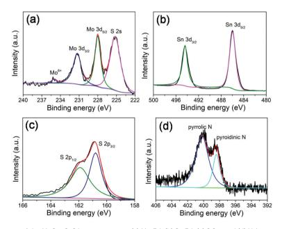
Fig. 3 High-resolution XPS spectra of the  $MoS_2@SnS$  heterostructure. (a) Mo 3d; (b) Sn 3d; (c) S 2p; and (d) N 1s spectra.
