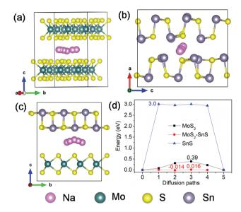
Fig. 9 Possible diffusion pathways of Na in (a) MoS<sub>2</sub>, (b) SnS supercells and (c) MoS<sub>2</sub>@SnS heterostructure, and (d) the corresponding energy barriers for Na diffusion in MoS<sub>2</sub>, SnS and MoS<sub>2</sub>@SnS.
