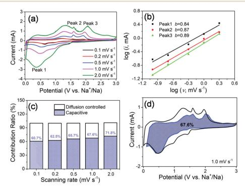
Fig. 7 (a) CV curves at various scan rates ranging from 0.1 to 2.0 mV s<sup>-1</sup>; (b) plots of log(i) vs. log(v) at the sharp cathodic/anodic peak pair (peak current: i, scanning rate: v); (c) capacity contributions at different scan rates; and (d) capacitive charge storage contribution at a scan rate of 1.0 mV s<sup>-1</sup>. The estimated pseudocapacitance contribution is shown in the blue region.
