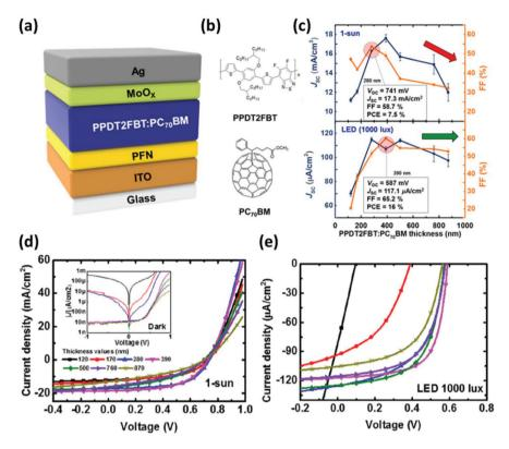
Fig. 5 Active layer thickness effect under 1 sun and LED illumination. (a) The device architecture and (b) molecular structures of PPDT2FBT and PC<sub>71</sub>BM. (c) Active layer thickness dependent  $J_{SC}$  and FF under 1 sun and LED illumination. J-V characteristics with various photoactive layer thicknesses under (d) AM 1.5G and (e) LED (1000 lx) illumination. (Inset of (d): dark J-V curves.) Reproduced from ref. 47 with permission from Elsevier.
