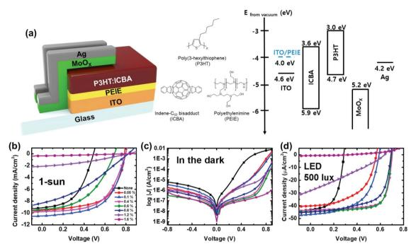
Fig. 6 PEIE thickness effect under LED illumination. (a) Device architecture, molecular structures of P3HT, ICBA and PEIE, and corresponding energy band diagram. *J*–*V* characteristics measured under (b) AM 1.5G illumination, (c) darkness and (d) LED (500 lx) illumination. Reproduced from ref. 52 with permission from Elsevier.
