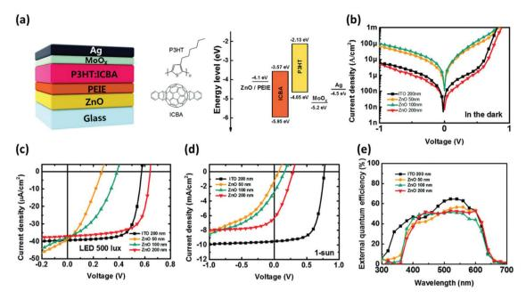
Fig. 7 Anode-free OPV devices. (a) Device structure of anode-free OPVs and the corresponding energy band diagram. *J*–*V* characteristics with ITO and ZnO electrodes (with different thicknesses of 50, 100 and 200 nm) under (b) darkness, (c) 500 lx LED and (d) AM 1.5G illumination. (e) Corresponding EQE spectra. Reproduced from ref. 54 with permission from The Royal Society of Chemistry.
