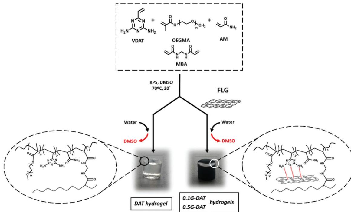
Fig. 1 Synthesis of DAT and G-DAT hydrogels.
