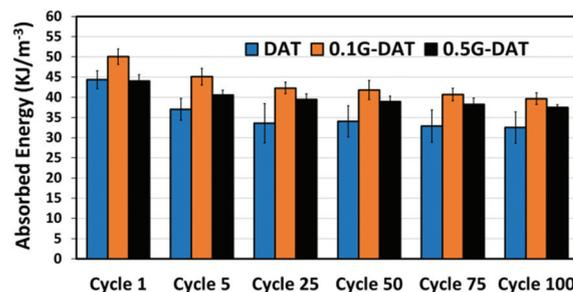
Fig. 7 100 cycle fatigue test for (G)-DAT hydrogels.
