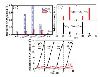
Fig. 6 (a) Photocatalytic  $CO_2$  reduction performances of all samples. (b) CO and  $CH_4$  mass spectra of C-ZNNS60. (c) Cyclic  $CO_2$  reduction curves for CO and  $CH_4$  yield (350 W, NaHCO $_3$  = 1 mmol).
