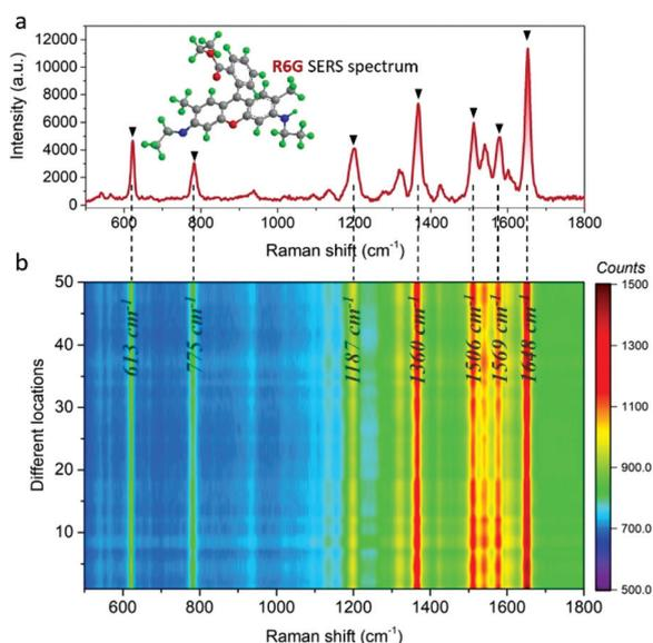
**Fig. 4** (a) Average SERS spectra measured from the R6G-treated 3D Ag hybrid nanostructure under the excitation laser wavelength of 473 nm. The concentration of R6G used in the measurement is  $10^{-7}$  M. (b) SERS contour plot of R6G ( $10^{-7}$  M) on the R6G-treated 3D-Ag-HNA substrate at 50 different locations.
