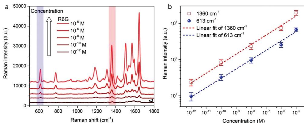
**Fig. 6** (a) The Raman spectra of R6G with different concentrations adhered on the 3D-Ag-HNA SERS substrate, and in order to be clarified, the spectrum of  $10^{-12}$  M R6G was multiplied by 2 fold. (b) The SERS intensity of R6G peaks at  $613 \text{ cm}^{-1}$  and  $1360 \text{ cm}^{-1}$  on 3D-Ag HNA as a function of the molecular concentration, on a log scale.
