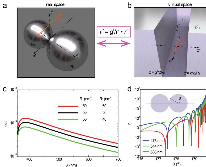
**Fig. 8** Theoretical analysis for the broadband enhancement of the nanoparticles with kissing points. (a) Schematic of a pair of nanoparticles with a point contact in real space. (b) The metal–insulator–metal structure can be achieved by coordinate transformation from real to virtual space. (c) The absorption cross-section  $\sigma_{\text{abs}}$  with different values of  $R_1$  and  $R_2$ . (d) The field enhancement  $\eta$  at three different wavelengths used in SERS measurement.
