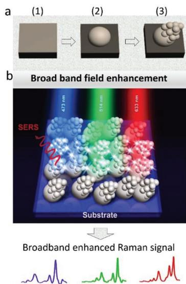
**Fig. 1** (a) Schematic illustration of the fabrication process for 3D Ag hybrid nanostructures: (1) deposition of Ag thin films; (2) solid state dewetting process; (3) oblique cluster beam deposition. (b) Cartoon of the 3D-AgHNA structure for broadband SERS detection.
