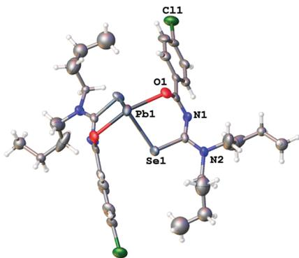
Fig. 4 Molecular structure of **2a**. Thermal ellipsoids are drawn at the 50% probability level. Only one part of the disordered <sup>t</sup>Bu chains is shown.
