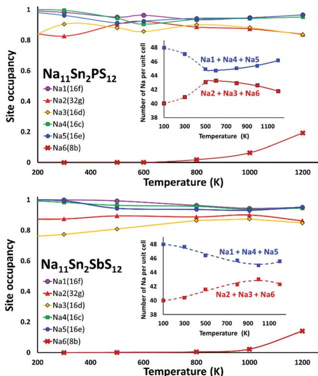
Fig. 8 Variation of the site occupancy factors of the different Na sites in Na<sub>11</sub>Sn<sub>2</sub>PS<sub>12</sub> (top) or Na<sub>11</sub>Sn<sub>2</sub>SbS<sub>12</sub> (bottom) over the temperature range 300 K to 1200 K. The respective insets display the same data as number of Na on the two groups of sites, *i.e.* the Na<sub>2</sub>–Na<sub>3</sub>–Na<sub>6</sub> site cluster and the Na<sub>1</sub>–Na<sub>4</sub>–Na<sub>5</sub> group of interconnecting sites.
