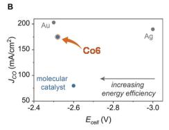
Fig. 12 Comparison of selectivity (A) and activity (B, partial current density) for CO production with Co6 inserted in a zero-gap membrane flow reactor and previous molecular and heterogeneous CO2 reduction electrocatalysts (adapted from ref. 118 with permission from AAAS, copyright 2019).
