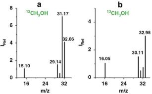
Fig. 15 GC/MS spectra and fragmentation pattern for the electrocatalyzed CO<sub>2</sub> conversion into CH<sub>3</sub>OH. Graphs show the mass fragmentation pattern of CH<sub>3</sub>OH (m/z 29 to 33) produced employing (a) <sup>12</sup>CO<sub>2</sub> or (b) 13CO2 as a reactant substrate. Reproduced with permission from ref. 250
