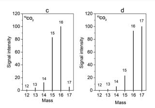
Fig. 16 Mass spectra labeling experiment demonstrating the carbon source for CH<sub>4</sub> production during CO<sub>2</sub> electrolysis, using Fe13 as a molecular precursor catalyst. Reproduced with permission from ref. 255. Copyright 2019, Wiley
