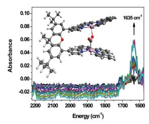
Fig. 14 Infrared spectro-electrochemistry data on a 1 mM solution of  $\text{Co}_2\text{3}$  in CH<sub>3</sub>CN (0.1 M  $^n\text{Bu}_4\text{NPF}_6$ , 0.5 M TEA) under CO<sub>2</sub> at potentials between -0.35 V and -0.85 V vs. Ag pseudo-reference. Inset: Calculated structure of the CO<sub>2</sub>-reduced complex adduct identified at 1635 cm $^{-1}$ . Adapted with permission from ref. 40. Copyright 2019, Springer Nature.
