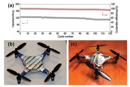
Fig. 23 (a) Cycling performance of the  $Zn/PZB-931/\gamma-MnO_2$  battery at 0.2C; (b) and (c) two different designs of  $Zn/\gamma-MnO_2$  battery pack as a replacement for the original device cover to supplement the main power source of unmanned aerial vehicles (UAVs). Reprinted with permission from ref. 397. Copyright 2019 American Chemical Society.
