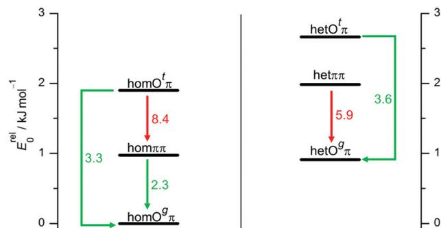
Fig. 6 Interconversion paths between **P** dimer structures including downhill barriers in  $\text{kJ mol}^{-1}$  at B3LYP-D3 level which are more (green) or less (red) feasible under supersonic jet expansion conditions.
