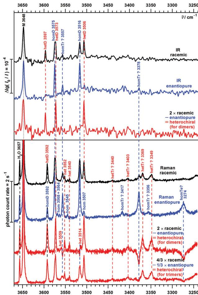
**Fig. 9** Experimental FTIR (top) and Raman (bottom) spectra of 1-phenylethanol P in the OH stretching range. The concentration in the Raman detected expansion is considerably higher. Bands are marked with the relative chirality of the monomers, in parts with the probable cluster size (M = monomer, D = dimers, Tr = trimers, Te = tetramers) and with their band position in cm<sup>-1</sup>.
