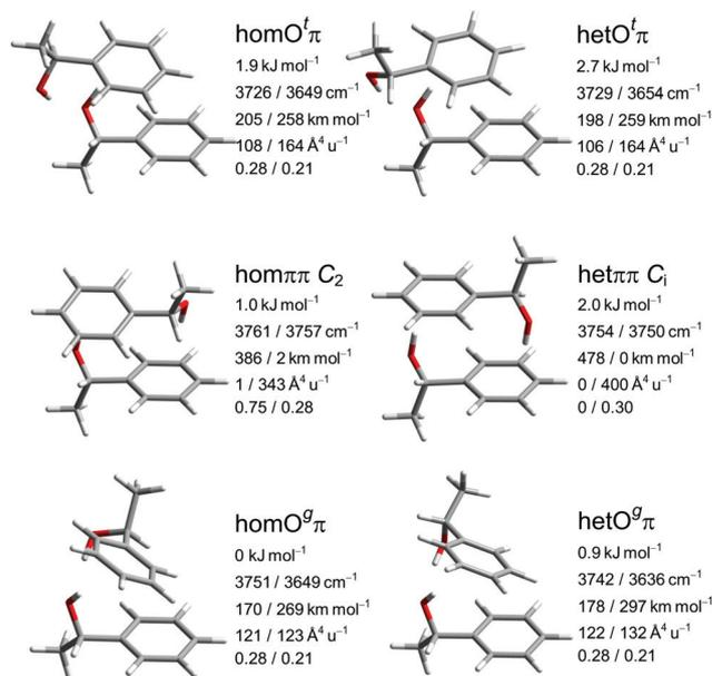
Fig. 5 Leading **P** dimer structures with harmonically zero-point-corrected relative energies, unscaled harmonic OH stretching wavenumbers, their IR intensities, Raman activities and depolarization ratios obtained at B3LYP-D3 level.
