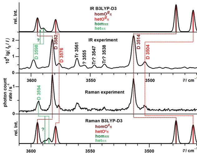
Fig. 8 **B** dimer B3LYP-D3 simulations (outer) compared to experimental IR and Raman jet spectra (inner traces) after shifting the harmonic OH stretching wavenumbers by  $-161.5 \text{ cm}^{-1}$  to match the monomer transition. A uniform conformational temperature of 100 K and a Gaussian FWHM of  $3 \text{ cm}^{-1}$  are assumed.
