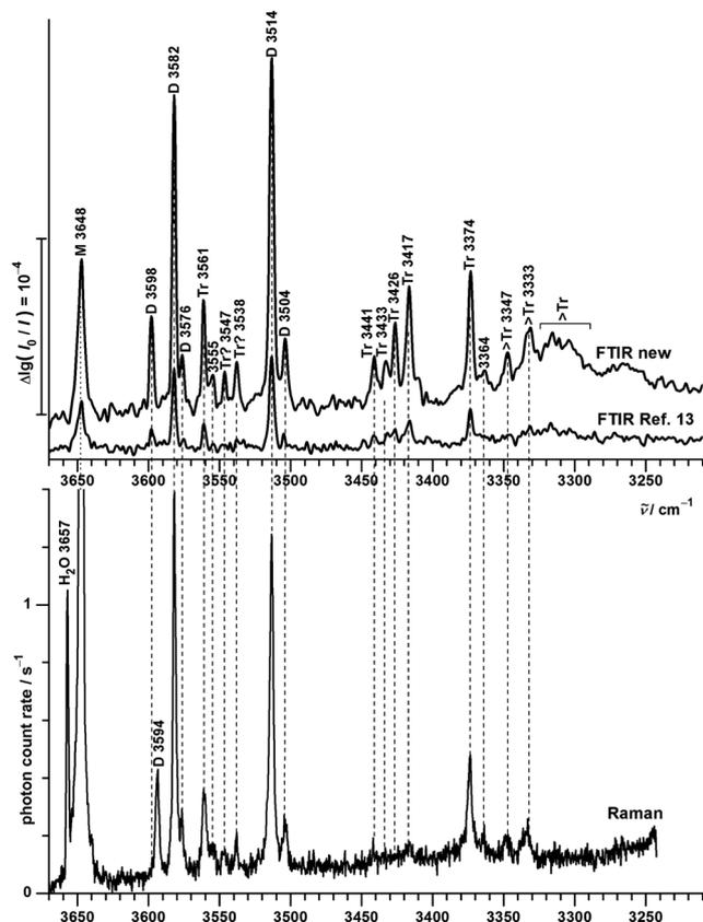
Fig. 7 OH stretching spectra of **B** seeded in helium from FTIR (upper traces, comparing new<sup>73</sup> (courtesy of M. Lange and E. Sennert) to published measurements<sup>13</sup>) and Raman (lowest trace, this work) spectroscopy. Cluster size assignments (M = monomers, D = dimers, Tr = trimers, >Tr = larger clusters according to previous<sup>13</sup> and this work) are labeled together with the wavenumbers of the band maxima.
