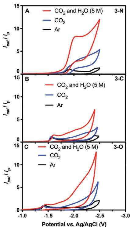
Fig. 1 CV scans of 0.5 mM solutions of **3-N** (A), **3-C** (B), and **3-O** (C) in DMF under argon (black), CO<sub>2</sub> (blue), and CO<sub>2</sub> with 5 M H<sub>2</sub>O (red).
