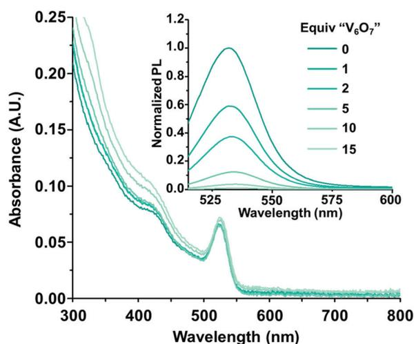
Fig. 2 The absorbance and photoluminescence (inset) spectra of CdSe–TOP with varying equivalents of  $[V_6O_7(OC_2H_5)_{12}]^{1-}$  (“ $V_6O_7$ ”). All samples contained 1  $\mu$ M CdSe with 0–15 equivalents of  $[V_6O_7(OC_2H_5)_{12}]^{1-}$  in dichloromethane and the photoluminescence was normalized to the absorbance at the excitation wavelength (500 nm).
