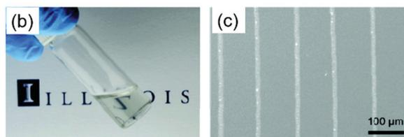
**Fig. 12** (a) Key constituents in the initial solution, ink, and printed features; (b) optical image of the silver ink in a scintillation vial; (c) conductive silver lines printed on a silicon substrate *via* direct-writing technology using a 100 nm nozzle. Reproduced with permission from ref. 45. Copyright 2012, American Chemical Society.
