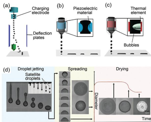
**Fig. 5** Inkjet printing principles: schematics of (a) CIJ, and DOD inkjet printing with (b) piezoelectric and (c) thermal head; (d) the complete inkjet printing process, showing the droplet jetting, spreading and drying stages. Reproduced with permission from ref. 98. Copyright 2018, Royal Society of Chemistry.
