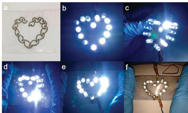
**Fig. 26** (a) Heart-like circuit drawn by a ballpoint pen; (b) 14 LED lights were lit to show a regular heart shape; LED lights can still work under different deformations; (c) outward bending; (d) inward bending; (e) stretching; and (f) flash photograph under stretching. Reproduced with permission from ref. 136. Copyright 2016, American Chemical Society.
