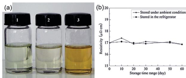
**Fig. 15** (a) Optical image of silver citrate particle-free inks: (1) freshly prepared; (2) preserved in the refrigerator for 60 days; (3) preserved under ambient conditions (25 °C) for 60 days; (b) variation of resistivity of printed patterns on a PET substrate cured at 150 °C for 50 min for different storage periods of the ink. Reproduced with permission from ref. 71. Copyright 2012 Elsevier.
