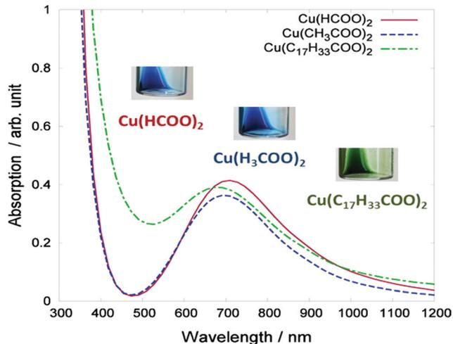
Fig. 7 Absorption spectra of the three types of copper complex ink: copper formate  $Cu(HCOO)_2$ , copper acetate  $Cu(CH_3COO)_2$ , and copper oleate  $Cu(C_{17}H_{33}COO)_2$ . The inset photographs display the visual color of the inks. Reproduced with permission from ref. 111. Copyright 2013, American Chemical Society.
