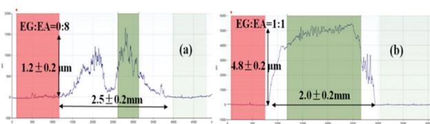
**Fig. 4** Surface profiles of a silver ink film after sintering: (a) coffee ring effect; (b) a flat film without the coffee ring using suitable solvent composition. Reproduced with permission from ref. 46. Copyright 2012, Royal Society of Chemistry.
