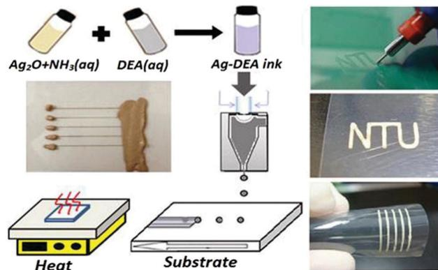
**Fig. 11** The formulation, deposition and metallization processes of the ink and the images of the written silver conductive films. Reproduced with permission from ref. 68. Copyright 2012, American Chemical Society.
