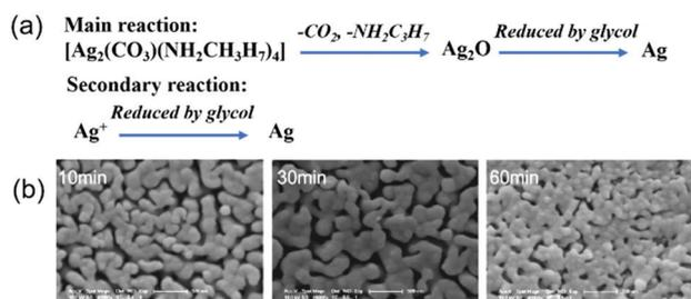
**Fig. 14** (a) Two main reaction mechanisms of the silver carbonate–amide complex ink during sintering; (b) SEM images of the conductive film sintered for 10, 30 and 60 minutes. Reproduced with permission from ref. 47. Copyright 2012, Royal Society of Chemistry.
