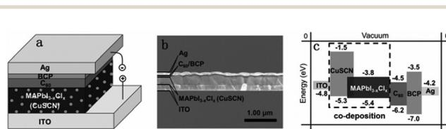
Fig. 9 (a) The schematic illustration and (b) cross-sectional SEM image of the hybrid perovskite/CuSCN device configuration; and (c) the energy level diagram of each layer in the device.<sup>96</sup>
