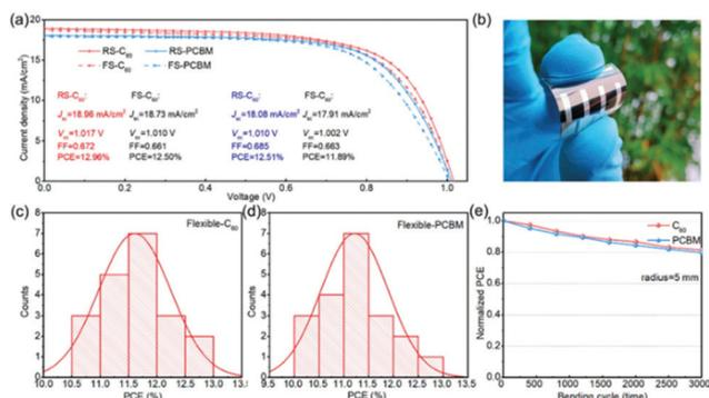
Fig. 17 (a) The  $J$ - $V$  curves of the best-performing flexible PSCs based on C<sub>60</sub> and PCBM ETLs, measured under both the reverse and forward scan direction; (b) image of the as-prepared flexible PSC; histograms of the PCE for 20 cells with (c) C<sub>60</sub> and (d) PCBM ETLs and (e) normalized PCE of the flexible PSC as a function of bending cycles with a radius of 5 mm.<sup>122</sup>
