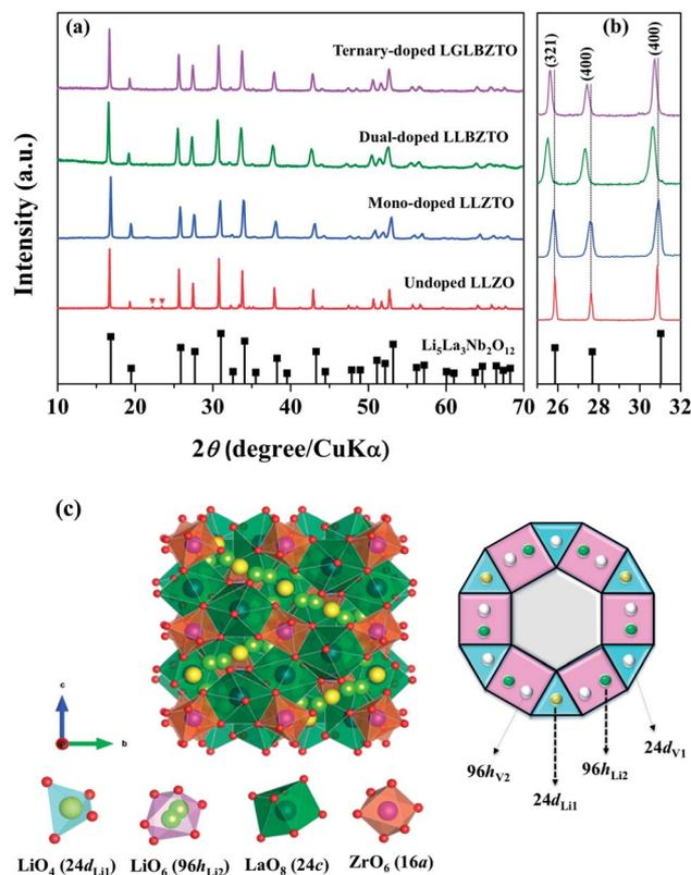
**Fig. 1** (a) XRD patterns and (b) peak shift of the undoped LLZO, mono-doped LLZTO, dual-doped LLBZTO, and ternary-doped LGLBZTO in the range of 25°–32°. (c) Crystal structure of cubic LLZO with the connectivity pattern of tetrahedral-24d<sub>Li1</sub> and 96h<sub>Li2</sub> cages projected on two dimensions.
