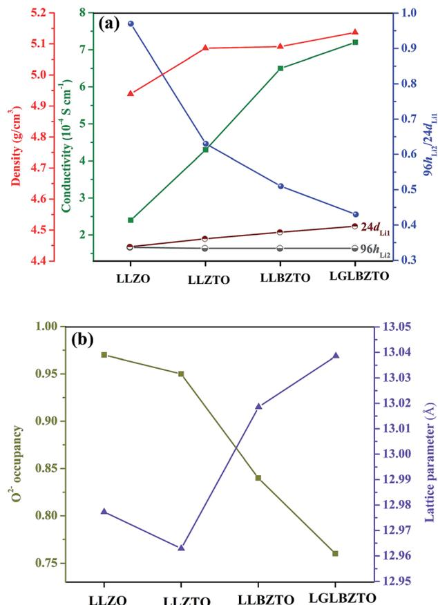
Fig. 5 Comparison plot for (a) density and total ionic conductivity at room temperature and Li occupancy ratio at  $96h_{\text{Li}2}/24d_{\text{Li}1}$ . (b)  $\text{O}^{2-}$  occupancy with lattice parameters of the undoped LLZO, mono-doped LLZTO, dual-doped LLBZTO, and ternary-doped LGLBZTO. The total ionic conductivity and density increase, whereas the Li occupancy ratio at  $96h_{\text{Li}2}/24d_{\text{Li}1}$  decreases with multi-ion doping into the garnet.
