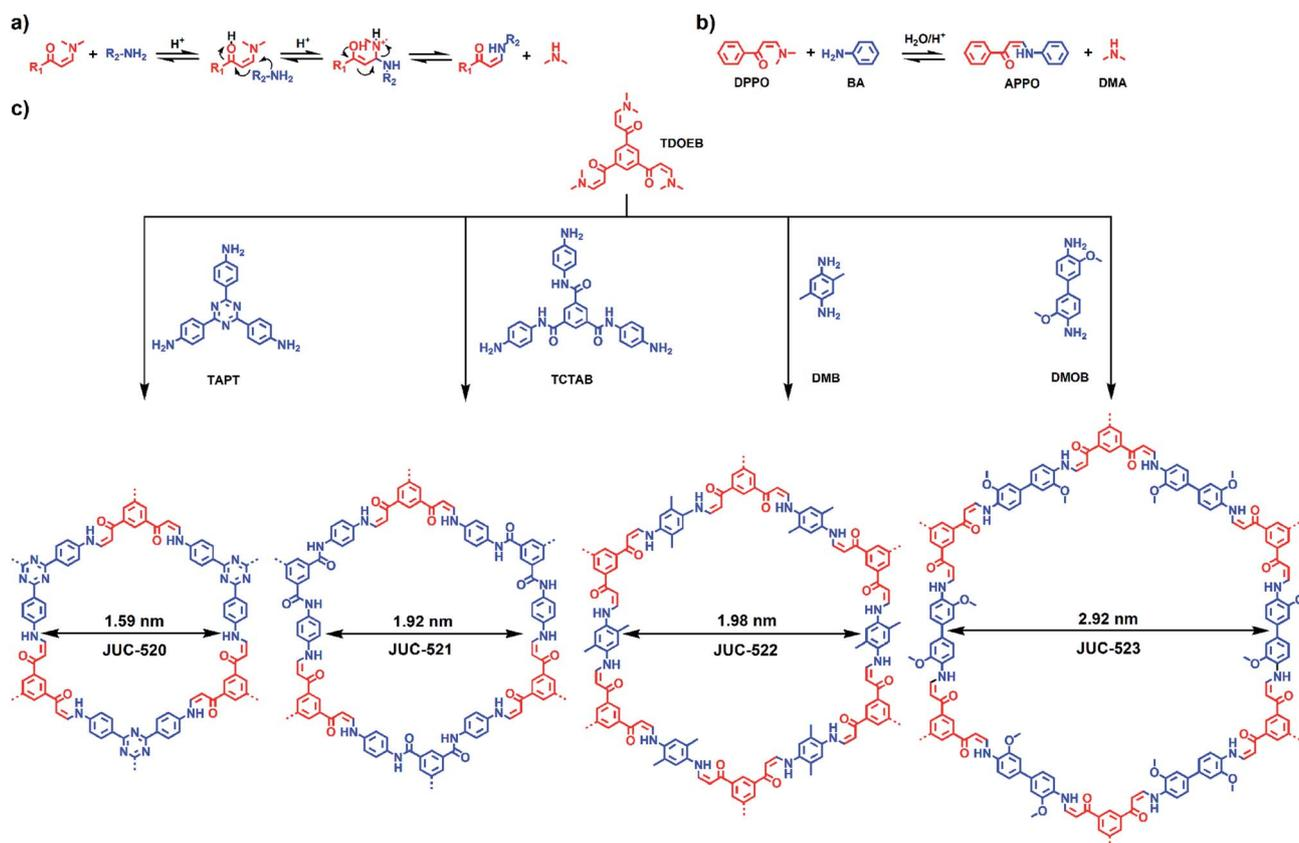
**Scheme 1** Strategy for ambient aqueous-phase synthesis of COFs. (a) Mechanistic pathway of the Michael addition–elimination reaction of  $\beta$ -ketoenamines and aromatic amines. (b) Model reaction between DPPO and BA to form APPO and DMA. (c) Condensation of TDOEB and TAPT, TCTAB, DMB or DMOB to give JUC-520, JUC-521, JUC-522 or JUC-523 with different pores.
