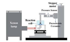
Fig. 6 Schematic diagram of the photoelectric-effect-accelerated ECNL instrument.
