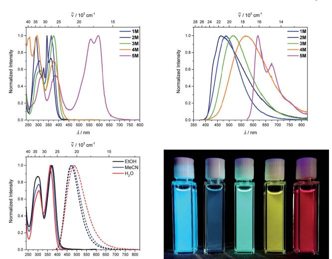
Fig. 3 Absorption (top, left) and emission spectra (top, right) of 1M-5M in water. Compound 2M was dissolved in 10% MeCN in water. Absorption and emission spectra of 1M in various solvents (EtOH: black, MeCN: blue,  $H_2O$ : red) (bottom, left) and picture of the solutions of 1M-5M in MeCN under UV irradiation.
