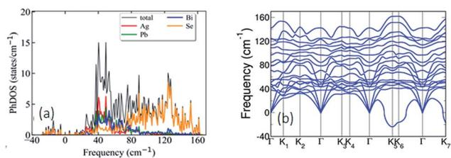
Fig. 4 (a) Atom projected phonon density of states reveals that low frequency optical modes ( $<50\text{ cm}^{-1}$ ) originate largely due to the vibrations of the Ag atoms followed by contributions from Pb and Bi atoms. (b) Phonon dispersion of  $\text{AgPbBiSe}_3$  showing that the acoustic branches have low cut-off frequencies ( $<50\text{ cm}^{-1}$ ).
