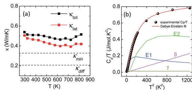
Fig. 2 (a) Total (black) and lattice (red) thermal conductivity of pristine  $\text{AgPbBiSe}_3$ . (b)  $C_p/T$  vs.  $T^2$  plot within the 2–30 K range. The red line is the fit produced using the combined Debye–Einstein model. The individual contributions from electronic ( $\gamma$ ), Debye ( $\beta$ ) and the two Einstein terms ( $E_1$  and  $E_2$ ) are also plotted.
