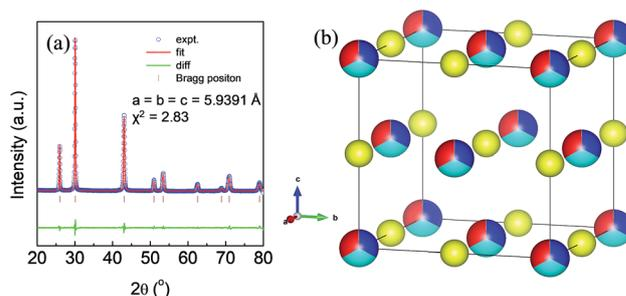
Fig. 1 (a) Le Bail refinement of the powder XRD pattern of  $\text{AgPbBiSe}_3$ . (b) Rock-salt structure of the compound  $\text{AgPbBiSe}_3$ . Red, sky blue, blue, and yellow atoms represent Ag, Pb, Bi and Se respectively.
