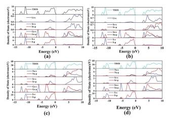
Fig. 5 Total and partial density of states (TDOS and PDOS) of title compounds: (a)  $Li_2SrGeS_4$ , (b)  $Li_2SrSnS_4$ , (c)  $Na_2SrGeS_4$ , and (d)  $Na_2SrSnS_4$ .
