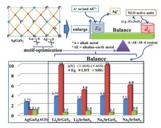
Fig. 6 Schematic diagram of designing new IR NLO materials by the motif-optimization with  $AgGaS_2$  as the template and title compounds achieve the suitable balance of wide  $E_q$  and good  $d_{ij}$ .
