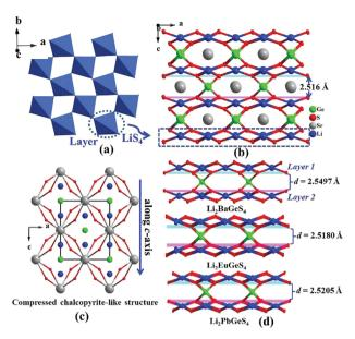
Fig. 1 (a) Corner-sharing (LiS<sub>4</sub>)<sub>n</sub> layer; (b) whole crystal structure of Li<sub>2</sub>SrGeS<sub>4</sub> (Sr–S bonds omitted for clarity); (c) 3D network structure composed of edge-sharing SrS<sub>8</sub> dodecahedra (Ge–S and Li–S bonds omitted for clarity); (d) comparison of the interlayer spacing between adjacent (LiS<sub>4</sub>)<sub>n</sub> layers in Li-based materials.
