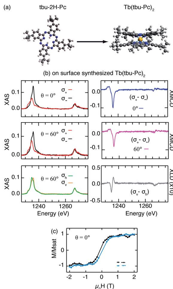
Fig. 5 (a) Schematic of *tbu-2H-Pc* and  $\text{Tb}(\text{tbu-Pc})_2$ . (b) XAS, XMCD, and XLD probed at the Tb  $M_{4,5}$  edges and (c) magnetization curve probed at the Tb  $M_5$  edge (3.7 ML *tbu-2H-Pc*/ $\text{Ag}(111)$  + 0.8 ML Tb;  $\mu_0 H = 50$  mT and 6.8 T for measurements with linear and circular polarizations, respectively,  $\mu_0 \dot{H} = 2$  T  $\text{min}^{-1}$  for magnetization curves measurements,  $T = 3$  K).
