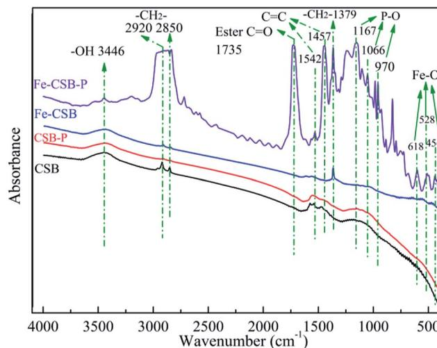
Fig. 7 FTIR spectrum of the CSB and Fe-CSB before and after adsorption.
