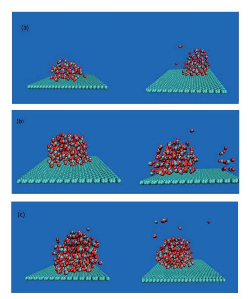
Fig. 2 Snapshot of bubbles under different systems. (a), (b) and (c) are bubbles formed by a system containing 60, 120 and 180  $CO_2$  molecules respectively, the left side is a bubble without an external electric field, and the right side is a bubble under an external electric field.
