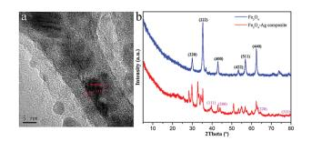
Fig. 4 HRTEM image of Ag nanowires (a) and XRD patterns of the  $Fe_3O_4$ -Ag nanocomposite (b).
