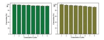
Fig. 8 Reusability test of the present Fe<sub>3</sub>O<sub>4</sub>-Ag nanocomposite as a catalyst for the reduction of 4-NP (a) and 2-NA (b) for eight consecutive cycles
