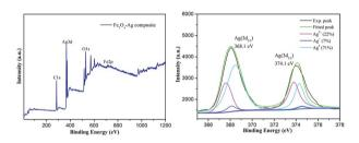
Fig. 6 XPS profiles of the  ${\rm Fe_3O_4-Ag}$  nanocomposite (a) and the deconvolution of Ag peaks (b).
