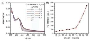
Fig. 7 (A) Absorption spectra of 10  $\mu$ mol L<sup>-1</sup> 2 upon the addition of Hg(II). (B) Job's plot data for evaluating the stoichiometry of the 2-Hg-2 complex. The total concentration of **2** and Hg(II) was kept at 20  $\mu$ mol L<sup>-1</sup>. 99% water/ DMSO (v/v) at pH 7.0 controlled by 10 mmol L<sup>-1</sup> Tris solution was used. Excitation and emission were performed at 368 nm and 445 nm, respectively.
