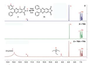
Fig. 10 <sup>1</sup>H-NMR spectra of 2 before and after the addition of excess TEA
