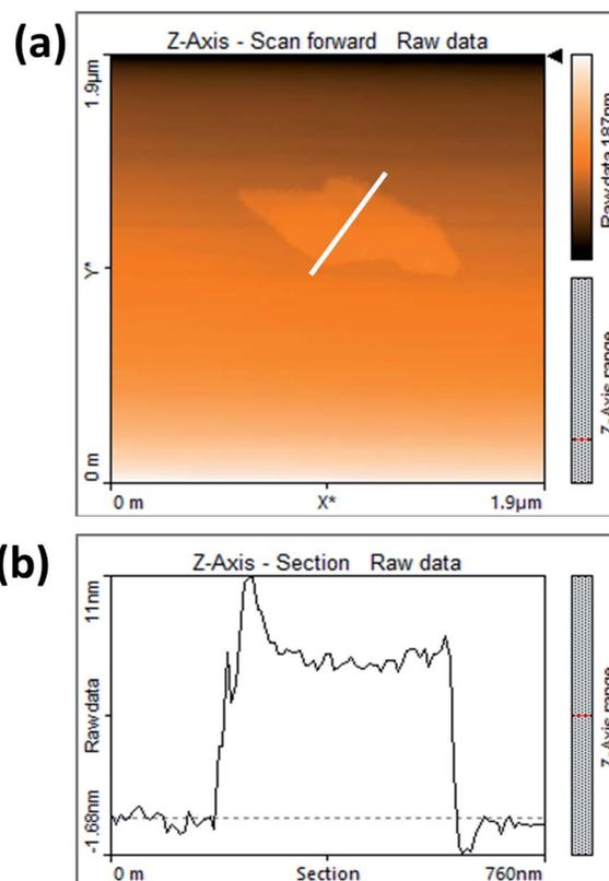
Fig. 3 (a) AFM image of MoS<sub>2</sub> nanosheets and (b) corresponding AFM height profile of MoS<sub>2</sub> nanosheets.
