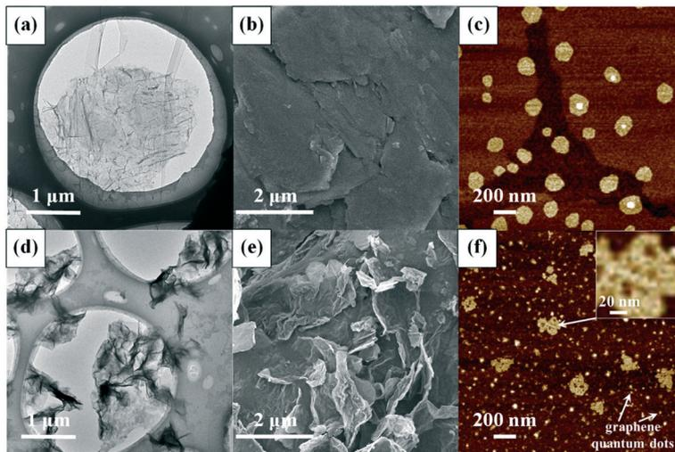
**Fig. 1** Morphology of graphene oxide: (a) transmission electron microscopy (TEM), (b) scanning electron microscopy (SEM), and (c) atomic force microscopy (AFM) images of pristine GO. Morphology of  $O_3$ -treated GO obtained *via* (d) TEM, (e) SEM, and (f) AFM.
