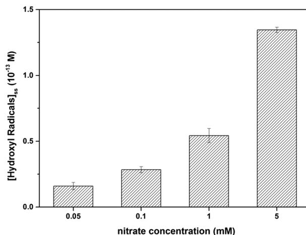
Fig. 5 Production of  $\cdot OH$  under UV irradiation of  $10 \text{ mg L}^{-1}$  GO suspension, as affected by the concentration of nitrate (0.05, 0.1, 1 and 5 mM), showing that the concentration of  $\cdot OH$  was dependent upon the nitrate concentration (the  $[\cdot OH]_{ss}$  generated in the system containing only GO was minimal and calibrated to zero).
