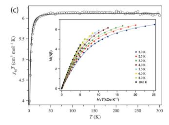
Fig. 5 Plots of  $\chi_{\rm M}T$  vs. T in the range 2–300 K in a 0.025 (T < 20 K) and 0.5 T ( $T \ge 20$  K) applied field and M vs. H/T (inset) for (a) 1, (b) 2, and (c) 3 in the 2-10 K temperature range. The solid lines are the best-fit curves, with the fit parameters given in Table 2
