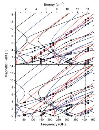
**Fig. 9** Field vs. frequency/energy map of turning points in complexes **1** (top) and **2** (bottom) at 10-15 K. Squares are experimental points; curves were simulated using spin Hamiltonian parameters as in Table 2. Red curves: turning points with magnetic field  $B_0$  parallel to the x-axis of the ZFS tensor; blue:  $B_0 \mid\mid y$ ; black:  $B_0 \mid\mid z$ . The two dashed vertical lines indicate the frequencies at which spectra shown in Fig. 6 were recorded.
