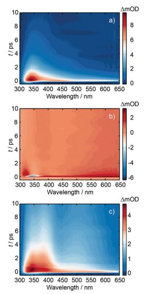
Fig. 4 273 nm pump and white light supercontinuum probe TA spectra for (a) dGMP, (b) dTMP and (c) d(GpT) aqueous solutions (pD 7) for delay times up to  $t \le 10$  ps. Note the different intensity scales used for each panel.
