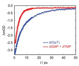
Fig. 7 Kinetics associated with the 1666 cm<sup>-1</sup> bleach feature for the mixture of mononucleotides (red open circles) and d(GpT) (blue open circles) upon 273 nm irradiation. Solid lines display the fits to experimental data (see Table 1 for fit parameters).
