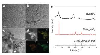
Fig. 2 (a) and (b) TEM images of manganese oxide nanoplates, (c) TEM image, (d) STEM image and EDS images of NMO NPs and (e) XRD patterns of NMO NPs and nanostructured P2-Na<sub>2/3</sub>MnO<sub>2</sub>.
