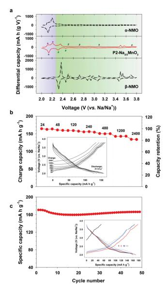
Fig. 4 Sodium storage performance of the nanostructured P2-Na<sub>2/3</sub>MnO<sub>2</sub>. (a) Differential capacity plots at 12 mA  $g^{-1}$ . Data for  $\alpha$ -NMO and  $\beta$ -NMO were adapted from ref. 32. (b) Rate performance at various charge current densities. (c) Cycling performance at 12 mA q<sup>-1</sup> (inset: corresponding voltage profiles).
