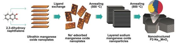
Fig. 1 Schematic illustration of the two-step method to synthesize nanostructured P2-Na<sub>2/3</sub>MnO<sub>2</sub>.
