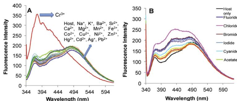
Fig. 9 Changes in the fluorescence spectrum of **10** (FONs) (20 M) in aqueous medium upon the (A) addition of 50 M of a particular metal nitrate salt in an aqueous medium and (B) addition of 50 M of a particular anion as tetrabutylammonium salt in an aqueous medium. Adapted with permission from ref. 32. Copyright 2015 Elsevier Ltd.
