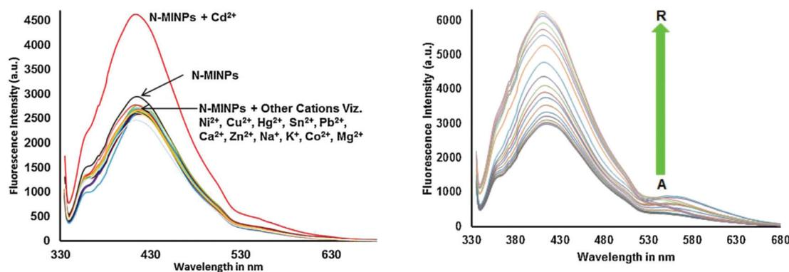
Fig. 11 Selectivity of **11** toward  $\text{Cd}^{2+}$  shows fluorescence enhancement as compared to other cations, and the fluorescence spectra of *N*-MNP suspension ( $1 \times 10^{-5} \text{ M}$ ) in the presence of different concentrations of  $\text{Cd}^{2+}$  ions. Adapted with permission from ref. 69. Copyright 2015 Elsevier Ltd.
