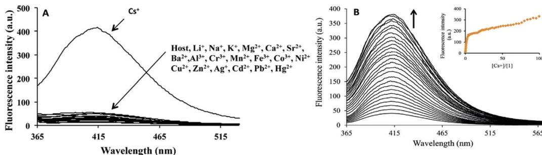
Fig. 22 (A) Changes in fluorescence spectrum of FONs of **30** (1.5 mM) in aqueous media upon the addition of 100 mM of a particular metal nitrate salt in the aqueous medium. (B) Changes in the fluorescence spectrum of FONs of **30** upon the successive addition of  $\text{Cs}^+$ ; inset shows the fluorescence intensity as a function of  $\text{Cs}^+$ . Adapted with permission from ref. 93. Copyright 2014 Elsevier Ltd.
