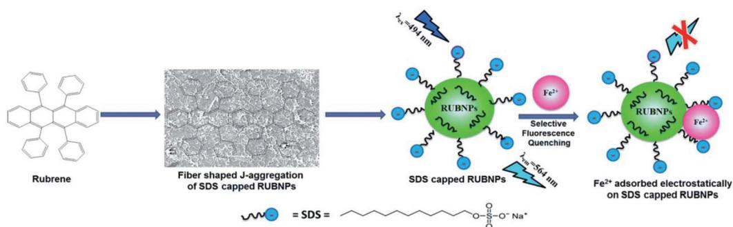
Fig. 18 Plausible fluorescence quenching mechanism based on  $\text{Fe}^{2+}$  ion adsorption on the surface of SDS-capped RUBNPs. Adapted with permission from ref. 86. Copyright 2015 the Royal Society of Chemistry.
