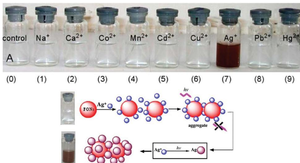
Fig. 3 Photographs of FON solutions after adding  $5 \times 10^{-4}$  M of the indicated metal ions after 24 h and the schematic illustration of the possible structure of Ag-nanoparticle-coated **3** aggregates. Adapted with permission from ref. 50. Copyright 2008 Elsevier Ltd.
