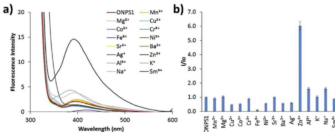
**Fig. 21** Fluorescence studies: metal ion binding test for nanoprobe **28** (0.1 mM) in an aqueous medium for the recognition of metal ions; (a) change in fluorescence spectra with respect to different metal ion additions; (b) relative fluorescence intensity at 410 nm against different metal ions. Adapted with permission from ref. 92. Copyright 2016 Elsevier Ltd.
