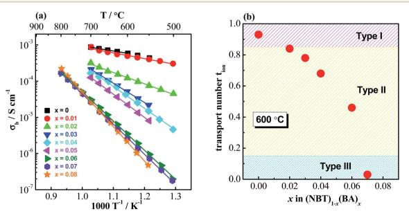
Fig. 7 (a) Arrhenius plots of the bulk conductivity and (b) oxide-ion transport number at 600 °C for the (NBT)<sub>1-x</sub>(BiAlO<sub>3</sub>)<sub>x</sub> ( $0 \le x \le 0.08$ ) solid solutions.48
