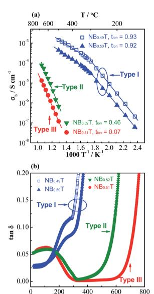
Fig. 1 (a) Arrhenius plot of bulk conductivity,  $\sigma_{\rm b}$  and (b) dielectric loss, tan  $\delta$ , at 1 MHz versus temperature for NBT with various A-site Bi nonstoichiometry:  $Na_{0.5}Bi_{0.49}TiO_{2.985}$ ,  $NB_{0.49}T$ ;  $Na_{0.5}Bi_{0.5}TiO_3$ ,  $NB_{0.50}T$ ;  $Na_{0.5}Bi_{0.51}TiO_{3.015}$ ,  $NB_{0.51}T$ ;  $Na_{0.5}Bi_{0.52}TiO_{3.03}$ ,  $NB_{0.52}T$ . Replotted after ref. 29
