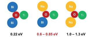
Fig. 3 Saddle-point configuration and associated activation energies for oxygen ion migration in NBT. Values taken from ref. 37.
