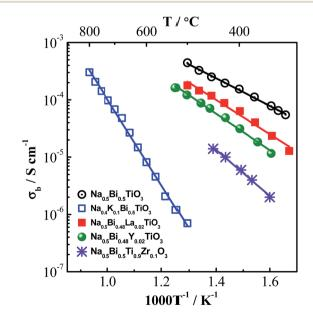
Fig. 4 Arrhenius plot of the bulk conductivity,  $\sigma_{\rm b}$ , of K-, Y-, La- and Zr-doped NBT.
