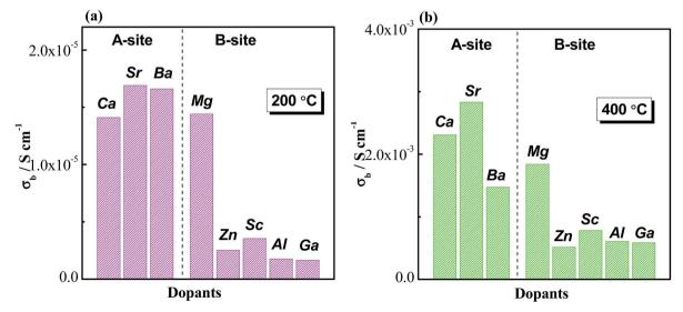
Comparison of bulk conductivity,  $\sigma_b$ , with A-site and B-site acceptor-dopants at (a) 200 °C and (b) 400 °C.
