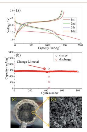
Fig. 5 The charge/discharge curves of the Li/S@pPAN cell from 1 V to 3 V at 1C (1C = 1675 mA  $\rm g^{-1}$ ) (a) and its cycling performance (b); the photo image (c) and SEM image (d) of the Li metal anode after 435 cycles of the Li–S@pPAN cell.
