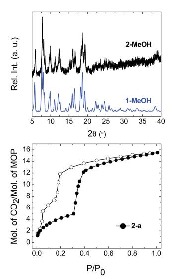
Fig. 7 (top) Comparison of the PXRD diffractograms for the flexible phase **1-MeOH** and the phase obtained for the Rh-containing MOP **2-MeOH**. (bottom)  $\rm CO_2$  sorption isotherms for **2-a**, measured at 195 K. Filled circles represent adsorption and empty symbols desorption.
