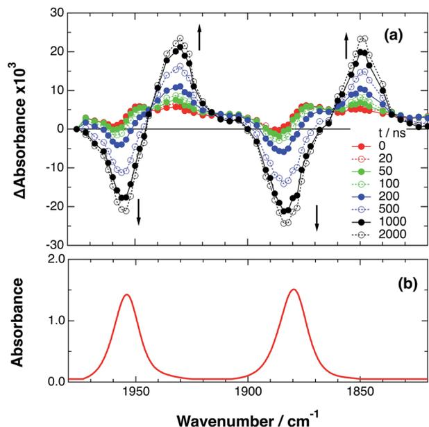
Fig. 3 (a) TRIR spectra (ns-system) recorded after 532 nm excitation of RuRe(OEt) (2 mM) in argon-saturated CH<sub>3</sub>CN/TEOA (5 : 1 v/v) containing 0.2 M BNAH. (b) FT-IR spectrum of RuRe(OEt) in CH<sub>3</sub>CN.
