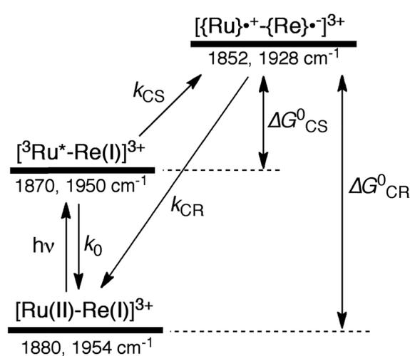
Scheme 2 Photoexcitation and the subsequent relaxation processes of a [Ru(II)–Re(I)]<sup>3+</sup> binuclear complex in the absence of any quencher molecules in solution, *i.e.*, the formation of a triplet metal-to-ligand charge transfer excited state ([<sup>3</sup>Ru\*–Re(I)]<sup>3+</sup>) followed by a charge-separated state ([{Ru}•+–{Re}•-]<sup>3+</sup>) due to electron transfer from the Ru unit to the Re unit. Wavenumber values shown are for the **RuRe(OEt)** complex.
