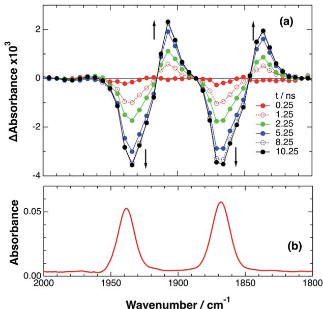
**Fig. 6** (a) TRIR spectra (ps-system) recorded after 532 nm excitation of  $\text{RuRe}(\text{FPh})$  (0.2 mM) in a DMF-TEOA (5 : 1 v/v) solution containing BIH (0.3 M), (b) FT-IR spectrum of  $\text{RuRe}(\text{FPh})$  in a DMF-TEOA (5 : 1 v/v) solution.
