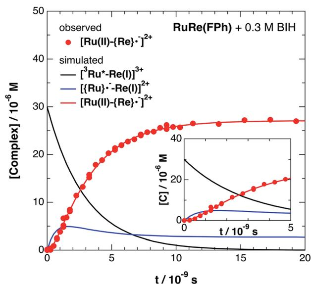
**Fig. 7** Time profile of  $[\text{Ru}(\text{II})-\{\text{Re}\}^{\bullet-}]^{2+}$  (●) in the ps-TRIR measurement of  $\text{RuRe}(\text{FPh})$  in the presence of 0.3 M BIH in an argon-saturated DMF-TEOA (5 : 1 v/v) solution after 532 nm excitation. The kinetic simulation results for  $[^3\text{Ru}^*-\text{Re}(\text{I})]^{3+}$ ,  $\{[\text{Ru}]^{\bullet-}-\text{Re}(\text{I})\}^{2+}$ , and  $[\text{Ru}(\text{II})-\{\text{Re}\}^{\bullet-}]^{2+}$  are also shown (solid lines).
