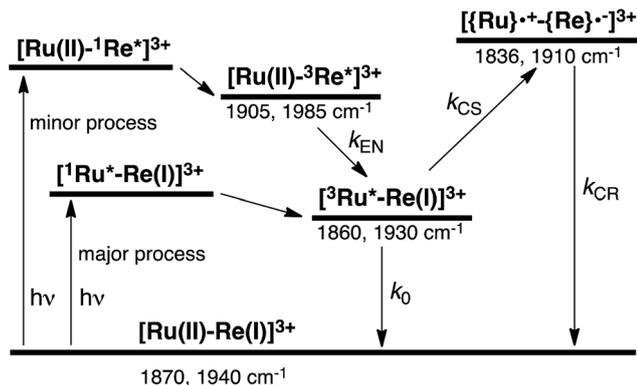
**Scheme 4** Photoexcitation and the subsequent relaxation processes of a  $[\text{Ru}(\text{II})-\text{Re}(\text{I})]^{3+}$  binuclear complex in the absence of any quencher molecules in solution, *i.e.*, the formation of a triplet metal-to-ligand charge transfer excited state ( $[^3\text{Ru}^*-\text{Re}(\text{I})]^{3+}$  and  $[\text{Ru}(\text{II})-^3\text{Re}^*]^{3+}$ ). Wavenumber values shown are for the  $\text{RuRe}(\text{FPh})$  complex.
