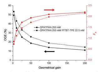
Fig. 4 Simulated OQE (black curves) and re-absorption number (red curves) of the LSC devices as a function of the geometric gain. The devices were based on 250 mM DPATPAN with (dashed line) or without (continuous line) PITBT-TPE in a PMMA thin-film matrix casted on a 1 mm thick square glass waveguide. The absorbance of all samples was set to 1.0 at 390 nm. All samples were excited at 390 nm and a total of 100,000 photons were traced in each simulation
