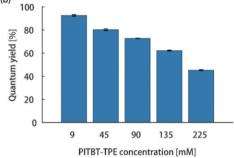
Fig. 2 (a) Normalized absorption and emission spectra of DPATPAN (250 mM in PMMA) and PITBT-TPE (200 mM in PMMA). (b) Emission quantum yield of PITBT-TPE at different concentrations in PMMA
