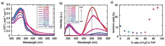
Fig. 2 Photophysical properties of TBFE in a THF/ $H_2O$  mixed solvent system. (a) Absorption spectra (1.0  $\times$  10<sup>-5</sup> M), (b) fluorescence spectra  $(1.0 \times 10^{-6} \text{ M}, \lambda_{\text{ex}} = 317 \text{ nm})$ , and (c) transition of photoluminescence quantum yield measured by the absolute method.
