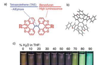
Fig. 1 Tetrakis(benzo[b]furyl)ethene (TBFE). (a) Molecular design. (b) Crystal structure showing twisting around the TAE centre (see ESI†). (c) Fluorescence intensity dependent on THF/H2O ratio (excitation at 365 nm).
