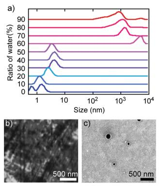
Fig. 3 Aggregation behaviour of TBFE. (a) Size distribution in THF/H<sub>2</sub>O solvents obtained by DLS measurements. This figure was obtained as a correlation function (Fig. S11, ESI†) and outputted as a volume distribution. (b and c) SEM images of TBFE on ITO formed by spin-coating using THF and THF/H<sub>2</sub>O = 10/90, respectively. The scale bars are 500 nm.
