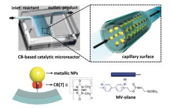
Fig. 1 Schematic illustration of a cucurbit[7]uril-based high-performance catalytic microreactor.
