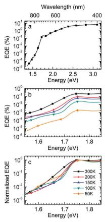
Fig. 3 (a) External quantum efficiency of MeLPPP: PCBM (1:1) bulk heterojunction devices measured at 300 K over the whole VIS-range down to the sub-bandgap region below 1.7 eV. (b) Temperature dependent EQE for MeLPPP: PCBM (1:1 by weight) blends in the range from room temperature (300 K) to 50 K, shown for the red spectral range. (c) EQE Spectra normalized to the S<sub>1</sub> transition peak of PCBM at about 1.76 eV.
