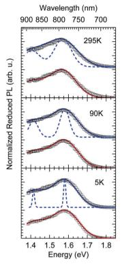
Fig. 8 Comparison of Franck-Condon-Fit (red line) and MLJ-Fit with (solid blue line) and without (dashed blue line) inhomogeneous broadening due to disorder for 295 K, 90 K and 5 K. Open symbols represent the measured data at distinct temperature. The parameters used in the fits are mentioned in the text
