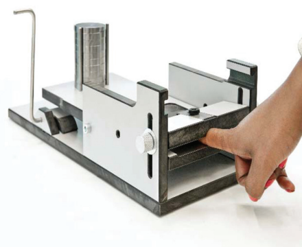
Fig. 1 Custom made fingerprinting device applied to maximize reproducibility in fingerprint deposition.
