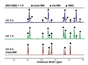
Fig. 3 <sup>1</sup>H NMR spectra of BM solutions with varied irradiation time.
