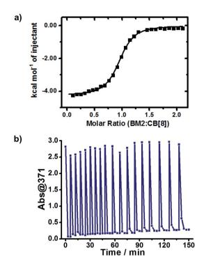
Fig. 5 (a) ITC data for the titration of the dimeric product (BM2) to CB [8]. (b) Diagram of Abs@371 *versus* irradiation time with continuous addition of BM for 18 cycles (initial concentration of BM was 0.5 mM).
