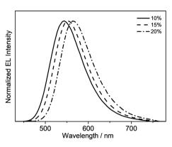
Fig. 6 Normalized EL spectra of solution-processable devices made from 8.
