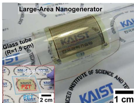
Fig. 21 Fabricated large-area thin PZT film NG on a curved glass tube. The inset shows a thin PZT film on a PET substrate formed by an LLO process.<sup>276</sup>
