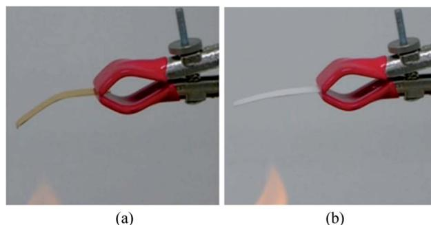
Fig. 17 Thermal stability of (a) paper-based nanogenerator and (b) polymer-based nanogenerator.<sup>245</sup>
