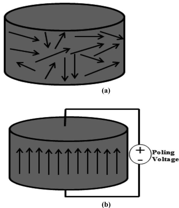
Fig. 16 (a) Before poling. (b) After poling.
