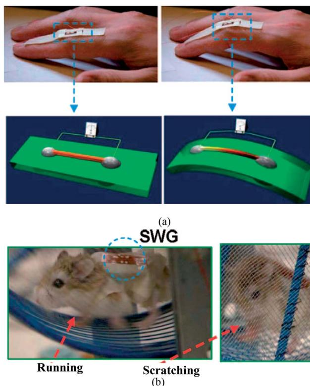
Fig. 20 Energy harvesting using an SWG from (a) an oscillating human index finger and (b) a live hamster.<sup>8</sup>
