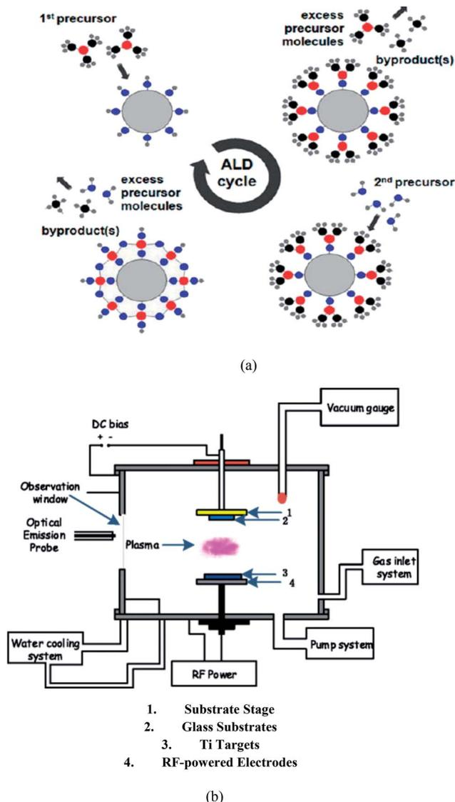
Fig. 11 Schematic representation of various seeding methods: (a) ALD<sup>93</sup> and (b) RF magnetron sputtering.<sup>94</sup>
