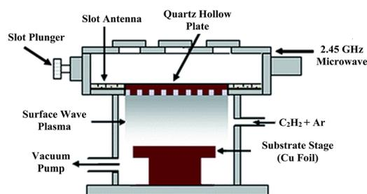
Fig. 7 Schematic of deposition of graphene film at low temperatures using a microwave-assisted surface-wave plasma chemical vapor deposition technique.<sup>58</sup>
