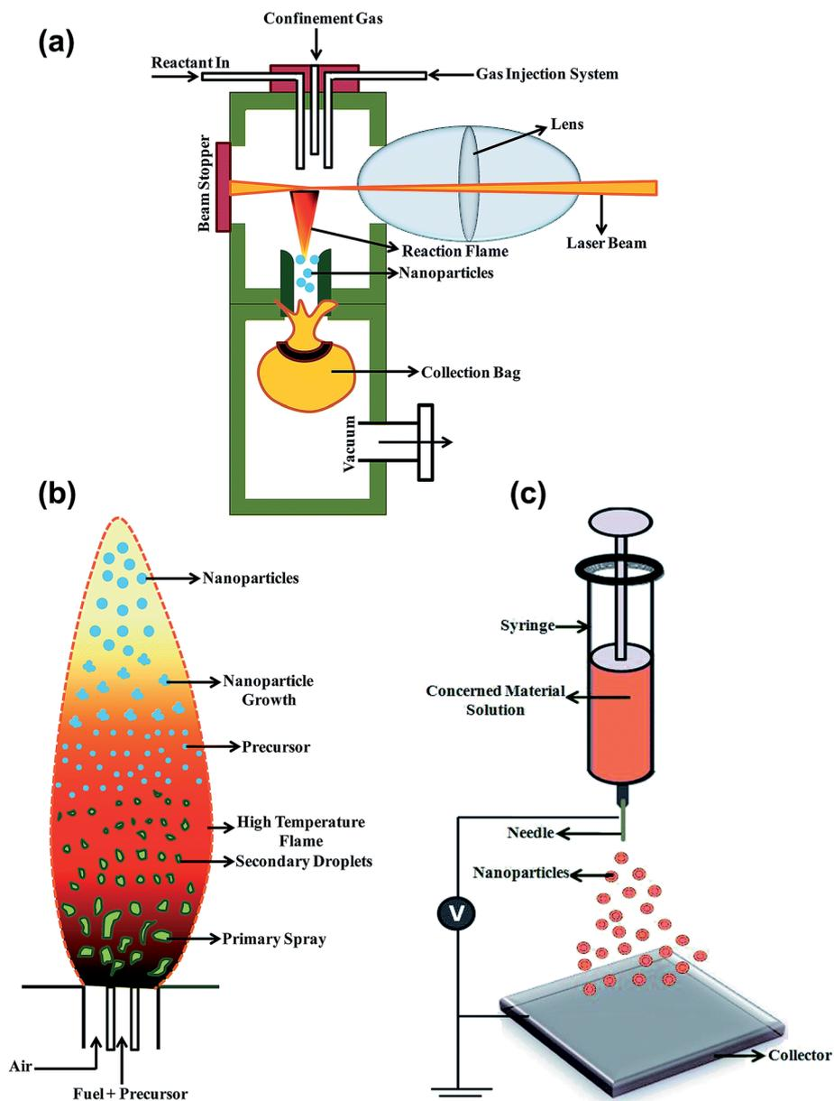
Fig. 10 Schematic diagrams of (a) laser pyrolysis, (b) flame spray pyrolysis and (c) an electrospaying technique for the synthesis of nanoparticles.<sup>80</sup>
