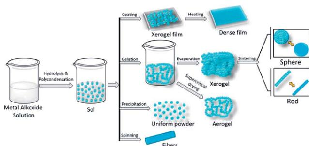
Fig. 9 Schematic illustration of sol-gel processes.<sup>75</sup>
