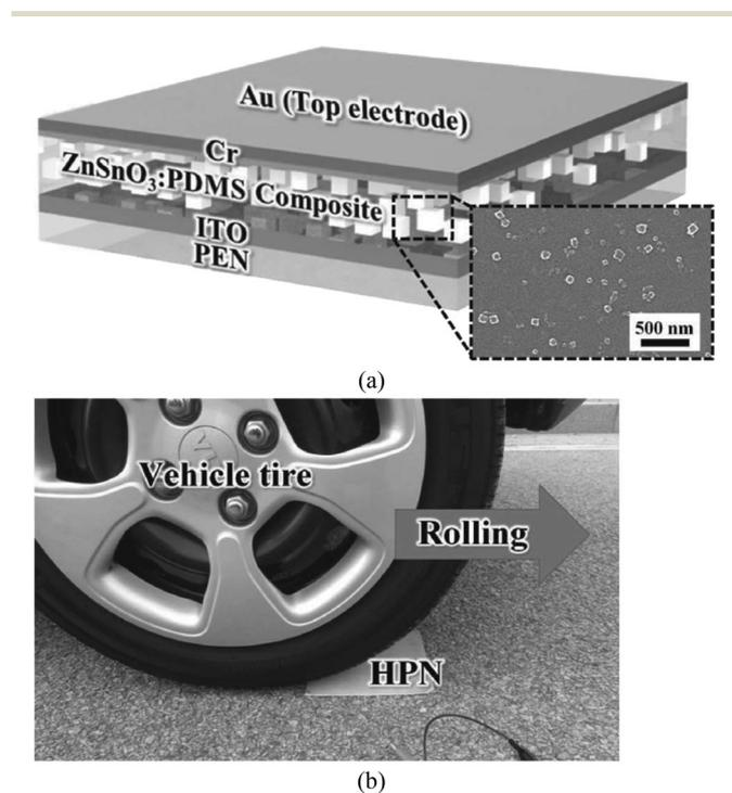
Fig. 18 (a) Schematic diagram of ZnSnO<sub>3</sub>:PDMS-based flexible hybrid PENG. (b) Experimental setup used for the generation of power from the hybrid PENG under a rolling vehicle tire.<sup>200</sup>
