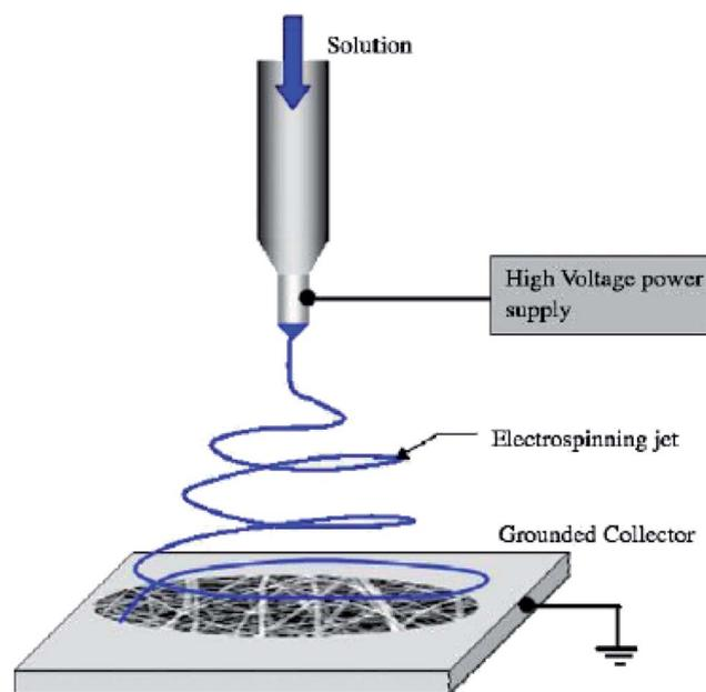
Fig. 13 Typical setup for electrospinning using a grounded collector.<sup>91</sup>
