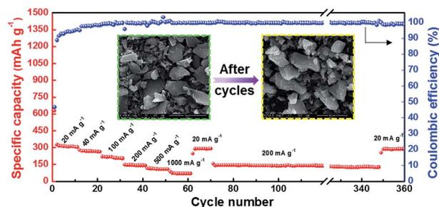
**Fig. 8** Discharge capacities of HC-1000 at different current densities of 20, 40, 100, 200, 500 and 1000 mA g<sup>-1</sup>, respectively. A long-term cycling performance is recorded from the 70<sup>th</sup> to the 350<sup>th</sup> cycles at 200 mA g<sup>-1</sup> and SEM images of the HC-1000 electrodes before and after 360 cycles.
