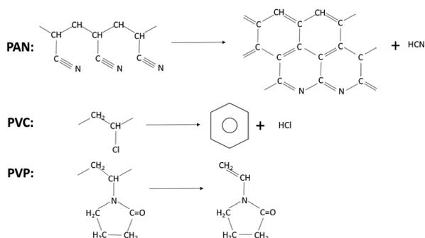
Scheme 1 The main products of PAN, PVC and PVP in pyrolysis process.
