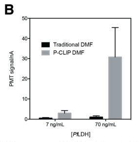
Fig. 5 DMF immunoassay for PfLDH. (A) Standard curve for PfLDH as determined by traditional DMF-ELISA. Error bars represent ± 1 std. dev. (n = 3). (B) Comparison of mean signals obtained by traditional DMF-ELISA (black) and P-CLIP modified DMF-ELISA (grey) for concentrations below the limit of detection (7 ng mL<sup>-1</sup>) and limit of quantitation (70 ng  $mL^{-1}$ ) of the traditional DMF-ELISA. Error bars  $\pm 1$  std. dev. (n = 3).
