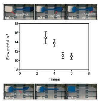
Fig. 2 Analysis of flow rate in P-CLIP virtual channels. Top and bottom: Video frames depicting six time-points during a P-CLIP imbibition of 75  $\mu$ L of PBS (with blue dye added to aid in visualization). Middle: Plot of flow rate measured as a function of time for the process (open circles). Error bars represent  $\pm$  1 std. dev. (n = 3).
