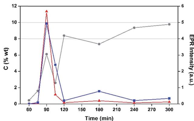
Fig. 4 Comparison of the radical content in the air deprived (red trace) and exposed (blue trace) samples derived from EPR signal intensity and the total C wt% (20% MeOH/Ar at  $260$  °C; gray trace) at various time intervals.
