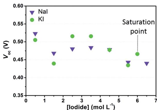
Fig. 3 Average  $V_{\text{oc}}$  values recorded one day after cell assembly.  $\text{I}_2$  was kept constant at 50 mM for all the cells. Data are referred to the 3<sup>rd</sup> measurement under 1 sun irradiation. Data referred to the electrolytes saturated with KI were arbitrarily placed at 6 M.
