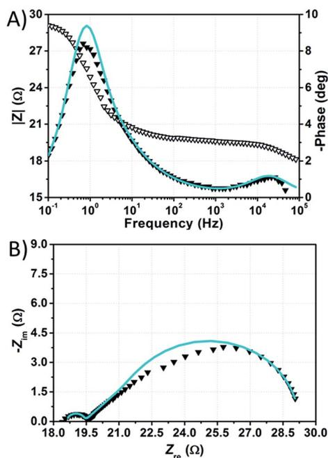
Fig. 8 Phase (filled triangles) and modulus (open triangles) Bode (A) and Nyquist (B) plots of the dummy cell filled with aqueous electrolyte comprised of NaI 1.50 M + I<sub>2</sub> 50 mM. Data points were fitted (light blue lines) according to eqn (1).
