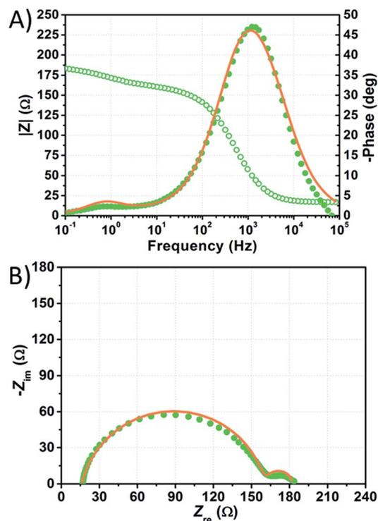
Fig. 9 Phase (filled circles) and modulus (open circles) Bode (A) and Nyquist (B) plots of the dummy cell filled with aqueous electrolyte comprised of KI 1.50 M + I<sub>2</sub> 50 mM. Data points, recorded five months after cell assembly, were fitted (lines) according to eqn (3) with the constraint  $R_{Pt} = 2$  Ω and  $C_{Pt} = 2 \times 10^{-5}$  F.
